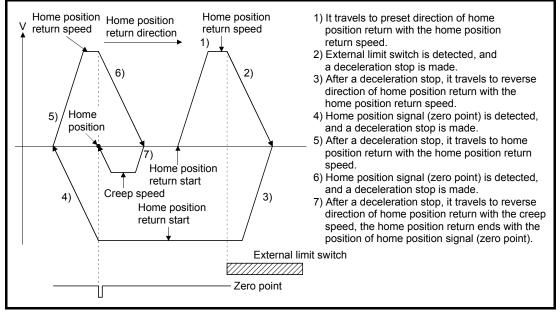
(b) When the zero point is not in the home position return direction.
