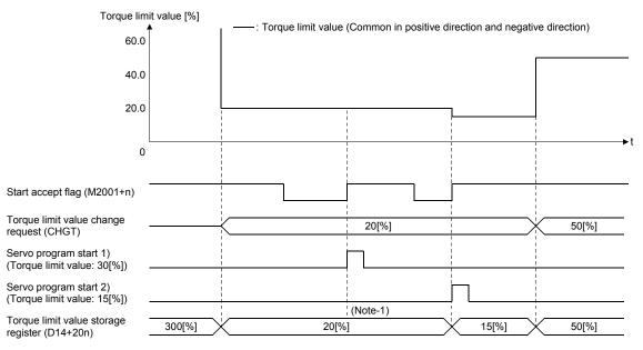
(Note-1): The torque limit value specified with servo program is cramped with the torque limit value changed by CHGT.
