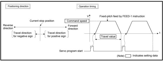
Fig.6.23 1 axis fixed-pitch feed control
