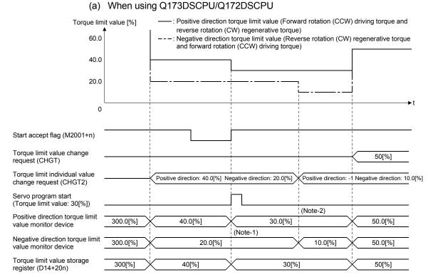
(Note-1): The torque limit value specified with servo program is cramped with the negative direction torque limit value changed by CHGT2.
