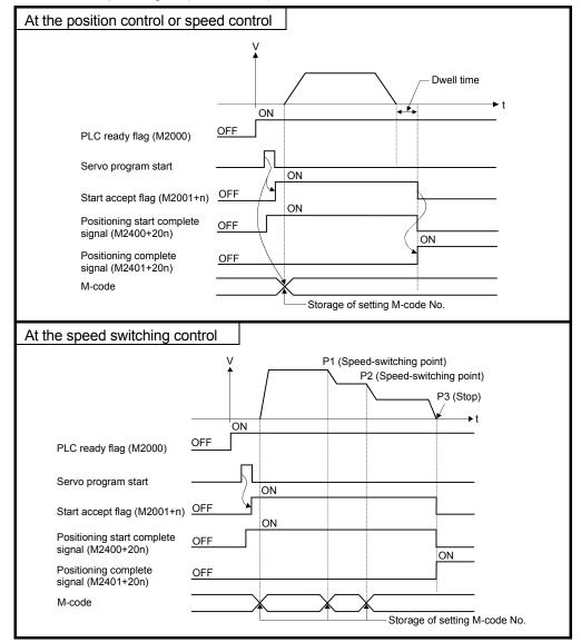
(c) When the M-code is read at positioning completion, use the positioning complete signal (M2401+20n) as the read command.
