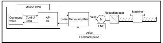
Fig. 4.1 Control content of the Motion CPU
