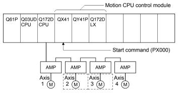
Speed-switching control of Axis 2 and Axis 3.
