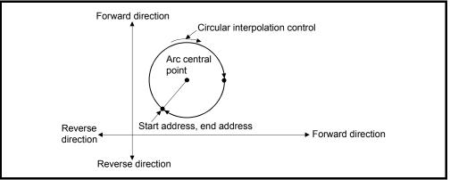
Fig.6.18 Positioning control of a complete round
