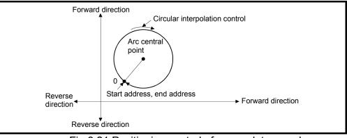
Fig.6.21 Positioning control of a complete round
