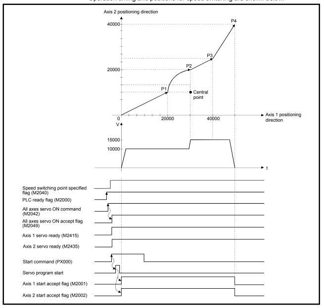
(3) Operation timing and speed-switching positions Operation timing and positions for speed switching are shown below.
