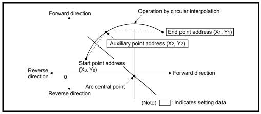
Fig.6.9 Circular interpolation control using absolute data method
