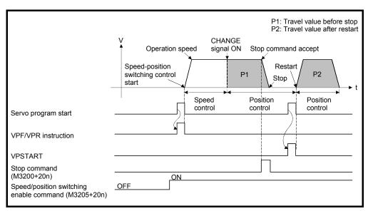
Fig.6.28 Re-starting during speed control
