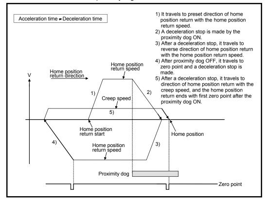
(d) When it starts in the proximity dog, the zero point is not passed (zero pass signal: M2406+20n OFF) at the time of the proximity dog is turned OFF during travel to reverse direction of home position return, it continues to travel with home position return speed until the zero point is passed. The zero point is passed again during deceleration by zero point pass, the home position becomes this side compared with the case to pass zero point at the time of the proximity dog OFF.
