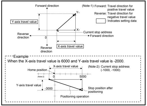
Fig.6.4 Positioning using incremental data method
