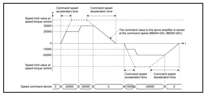
When the rotation direction is changed due to the command speed change during speed control, the operation is as follows.
