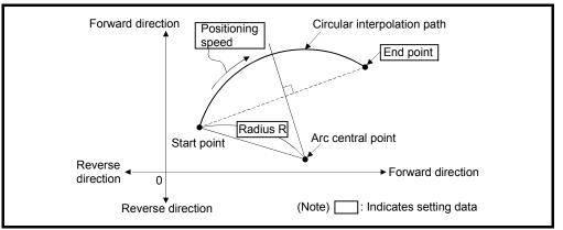
Fig.6.15 Circular interpolation control using incremental data method
