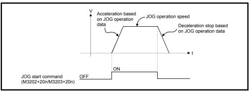
JOG operation for axis for which JOG start command is turning on is executed.
