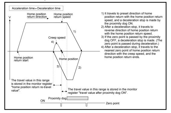
(e) If the zero point is passed during deceleration, the nearest zero point from deceleration stop position to home position return direction is set as the home position.
