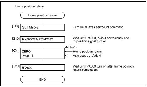
(Note-1): It is necessary to turn on the zero pass signal before execution of the home position return instruction for data set method home position return.
