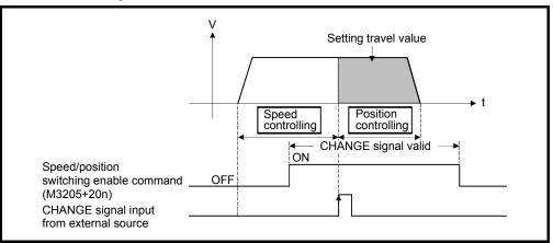
Fig. 6.27 Re-starting during speed control
