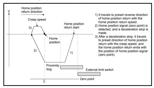
(e) If the zero point is passed during deceleration, the nearest position of home position signal (zero point) of home position return direction from deceleration stop position is set as the home position.
