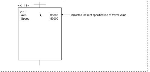
(b) The travel value is stored in the data register for travel value change during speed control in the Motion SFC program. When the CHANGE signal turns on, the contents of the data register for travel value change are set as the travel value.
