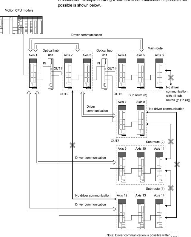
(a) Servo amplifier layout for driver communication
