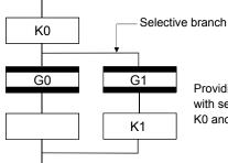
Providing transition G1 with cancel device condition specified with servo program K0 will cancel to execute of servo program K0 and allow servo program K1 to start.
