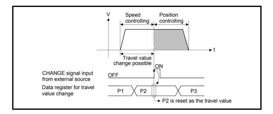
(5) Travel value area after proximity dog ON The travel value since the position mode was selected by the CHANGE signal input from external source is stored in the travel value after proximity dog ON storage register (D10+20n, D11+20n). [Cautions]
