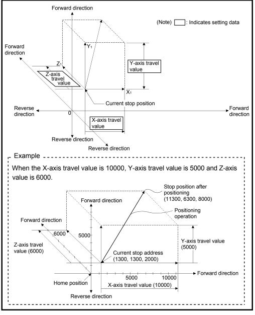
Fig.6.6 Positioning using incremental data method
