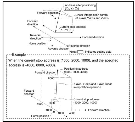
Fig.6.5 Positioning using absolute data method
