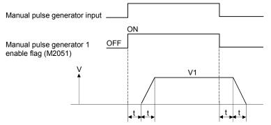
Output speed (V1) = [Number of input pulses/ms]  $\times$  [Manual pulse generator 1- pulse input magnification setting]
