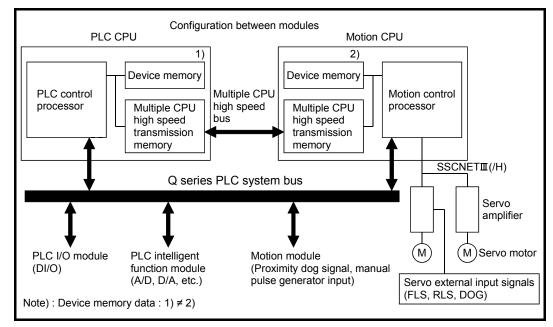
Fig.3.1 Flow of the internal signals/external signals
