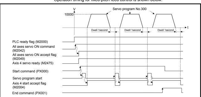
Operation timing for fixed-pitch feed control is shown below.
