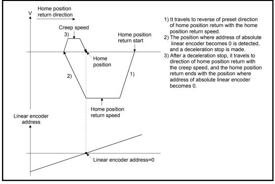
(b) When the position where address of absolute linear encoder becomes 0 is not in the home position return direction.
