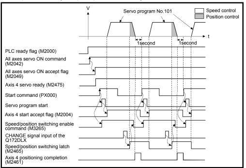
Operation timing for speed-position switching control is shown below.
